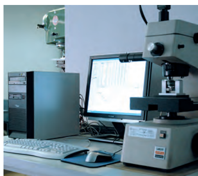
Automatic Hardness Tester to Vickers
