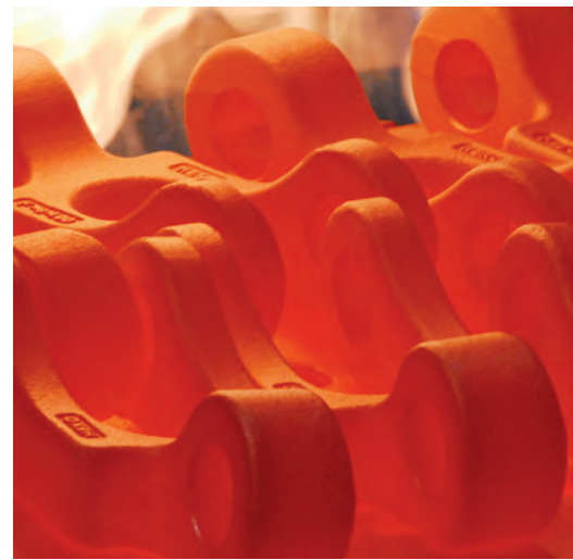
Quench and Temper of Forged Links
