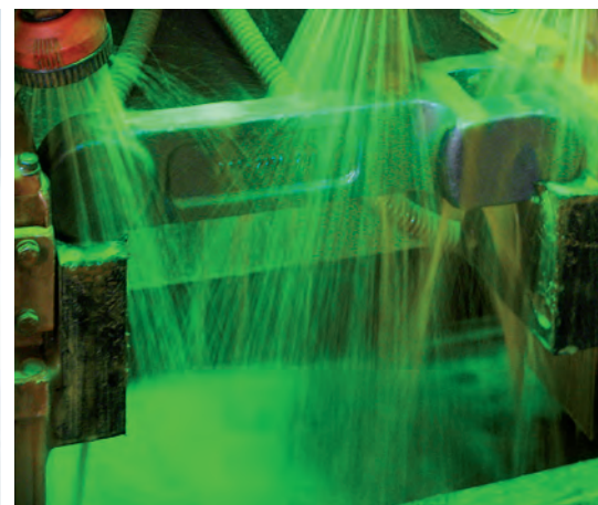
Magnetic Crack Testing of Forged Link
