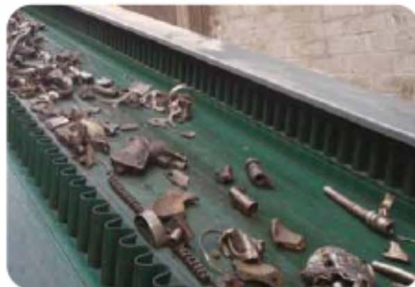
FRGZ-5mm with welded Sidewalls: METAL RECYCLING
