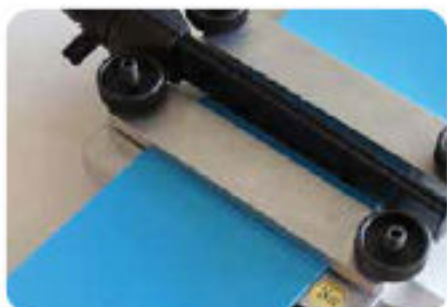
Welding narrow flat belts with Pliers P-200
